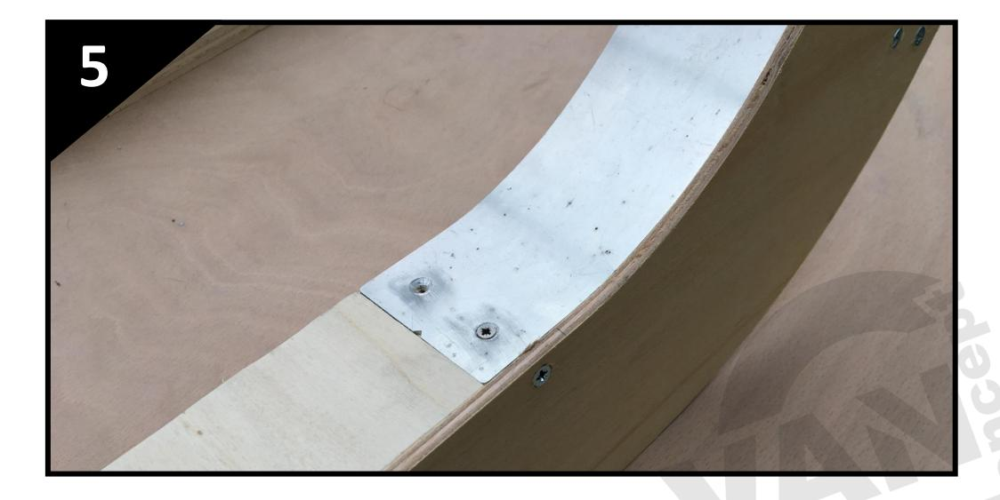
With the corner profile matching the plywood edge, take one of the smaller diameter screws and attach the metal to the plywood in the position shown.
