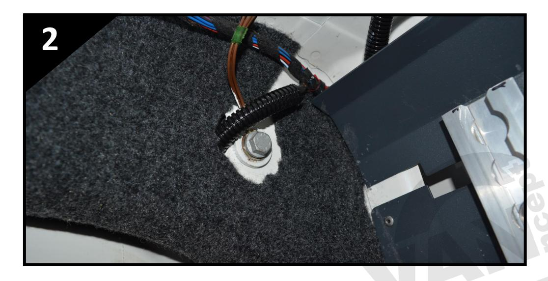
Line the van interior with chosen lining material around the earth point and use a pointed object the locate the holes.
