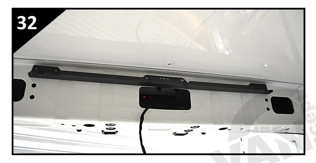
• At the rear, X6 can be fitted by aligning the bottom edge with the top of the OEM light cutout, and then drilling the four smaller 4.2mm holes either side and fitting 1x 4x8mm rivet in each hole.
