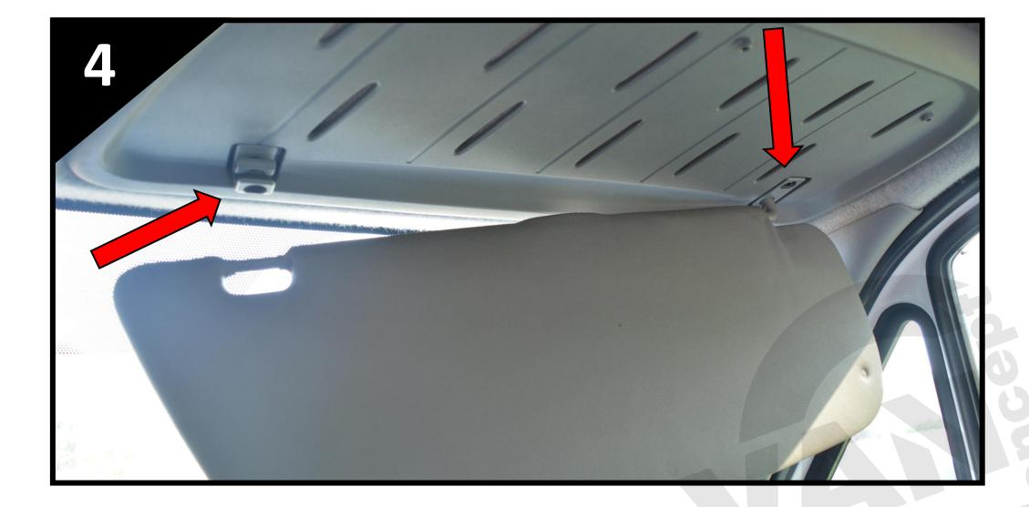
• Loosen the two remaining bolts that secure the sun visor and shelf.
