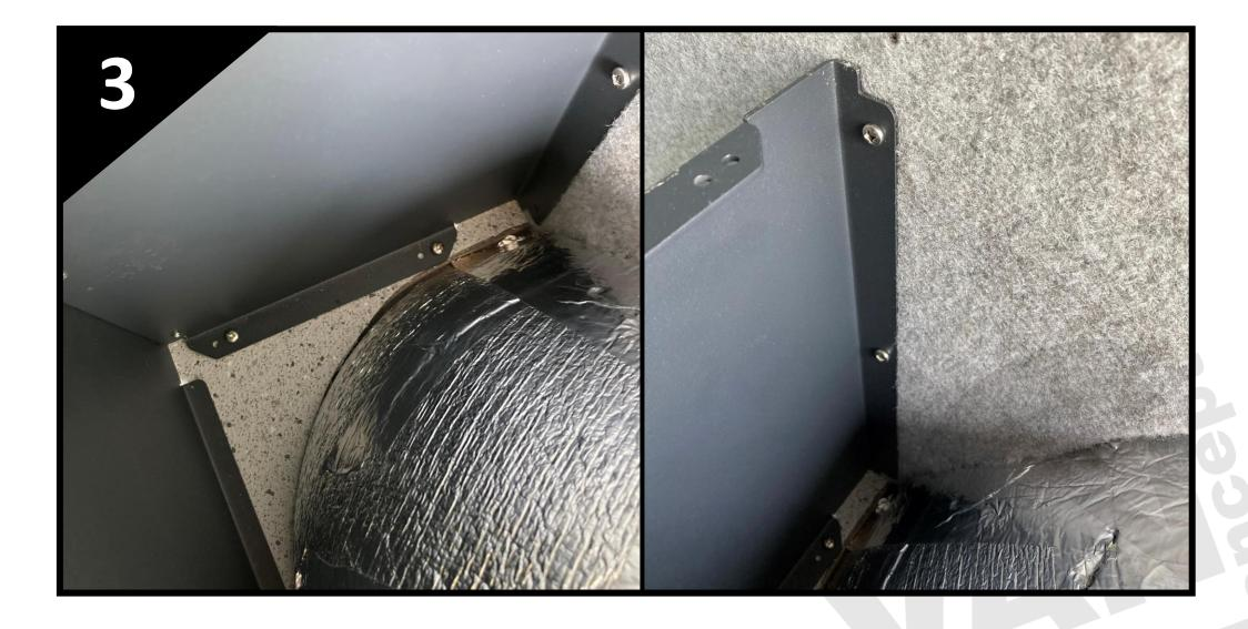
• Ensuring the Arch Box is square and the front panel fits, screw the end panels to the van floor using some more pan head screws.
