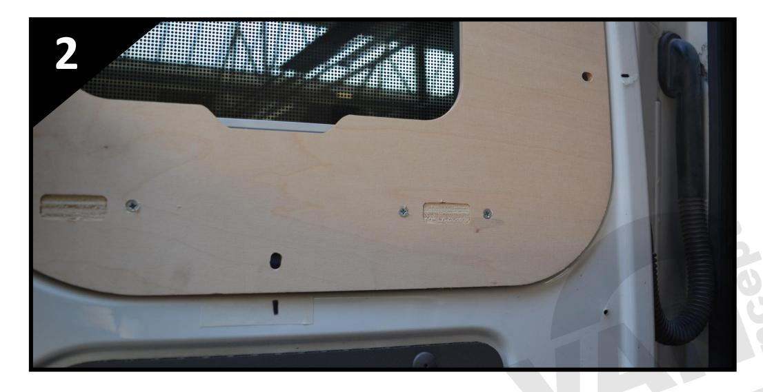
To locate the mounting brackets, mark out the position of the six brackets by creating a centreline on some masking tape from the mounting holes in the panel.
