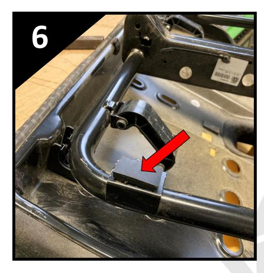
• If fitting to a VW Crafter '06-'17 & Mercedes Sprinter '06-'18 model van, apply the two selfadhesive rubber blocks to the flat area shown above on the underside of the seat frame.
