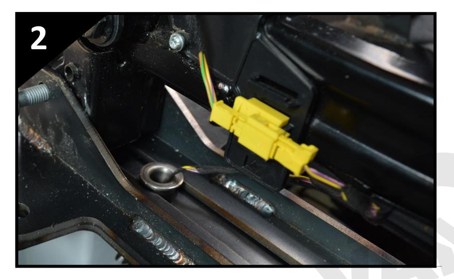
Disconnect the van battery and wait 20 minutes, before disconnecting the Airbag sensor connector mounted on
