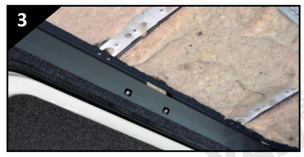
There are two sets of two holes machined into the sections at each roof rib position. This is to allow for variation in the positioning of the ribs. Choose one hole either side that best lines up and drill Ø4mm holes in the vans roof ribs, de-burr the hole and rivet the section in place. (We advise applying some anti-corrosion paint to the bare metal in the hole before fitting the rivets and to remove any metal swarf).
