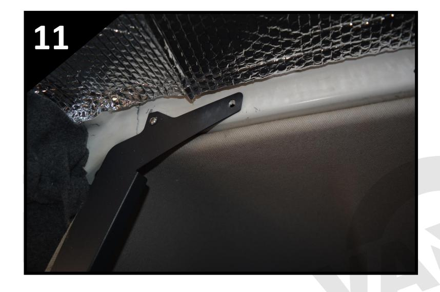
• If fitting the bulkhead shelf top with our Cab Headliner Shelf fitted, remove the M6 button head bolt on the left sided bracket, as shown.
