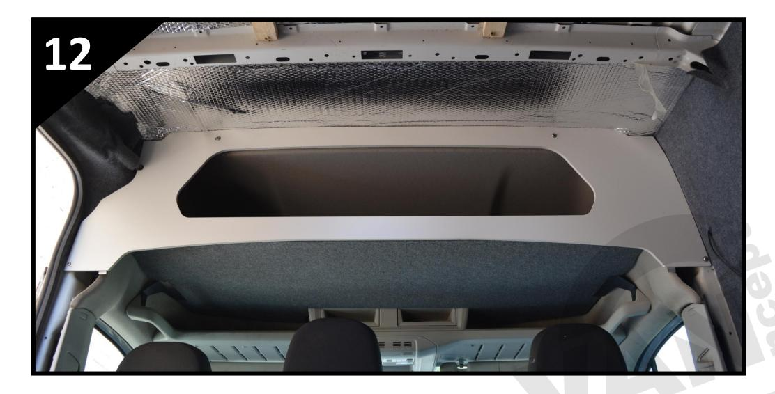
• Offer either top piece into place and fit the 4x M6x25mm flanged head bolts through the slots in the sides and top and bolt into the threaded holes in the metalwork.
