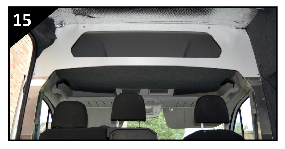
• If fitting the kit with our cab headliner shelf, equally space and screw the 5x 4x25mm CSK screws supplied with the shelf kit through the strengthening rib on the back edge of the shelf and into the reverse side of the bulkhead surround, to secure the two pieces together.
