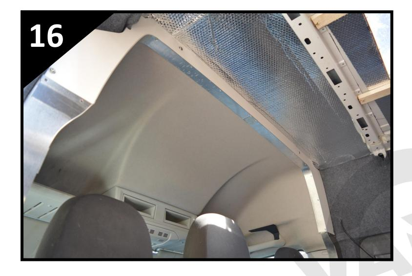
• With the open top fitted with the OEM head lining, the aluminium profile should neatly align with the edge.
