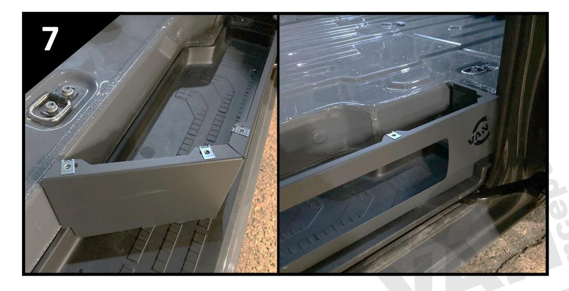
Fit the four M5 Chimney Nuts to the four slots on the top flange of the storage box. Note the flat side of the clip should be facing upwards.
