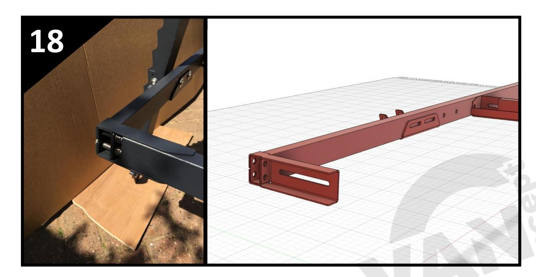
At the front, position both the Bed Frame Bracket Front brackets over the ends of the Side Beams (note orientation), before fitting 1x M8 x 40mm button head bolt, with 2x M8 washers and 1x M8 nyloc nut through each hole, on both brackets as shown, before tightening.
