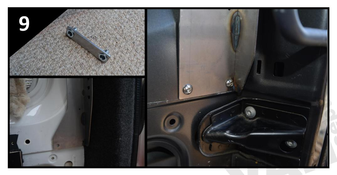
• The rear strut is correctly aligned when the bottom edge is parallel with the bodywork.
