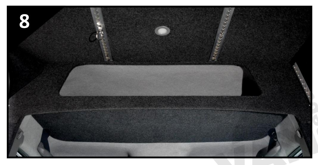
• If fitting the kit with our cab headliner shelf, equally space and screw the five long screws supplied with the shelf kit through the strengthening rib on the back edge of the shelf and into the reverse side of the bulkhead surround, to secure the two pieces together.
