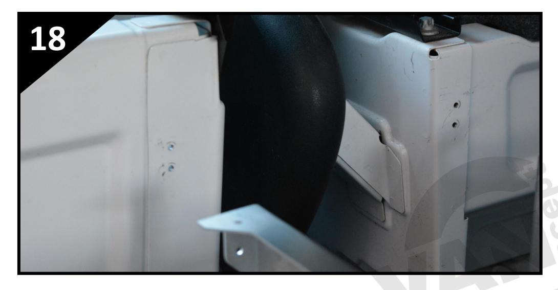
• Drill 8x Ø4mm holes in the seat bases where the bulkhead brackets holes have previously been marked and de-burr the holes (We advise applying some anti-corrosion paint to the bare metal in the hole before fitting the rivets).
