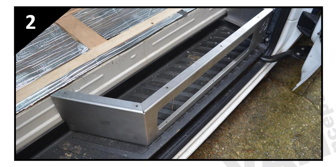
• Position the box on the step and mark/pre-drill Ø3mm holes in the side-step.
