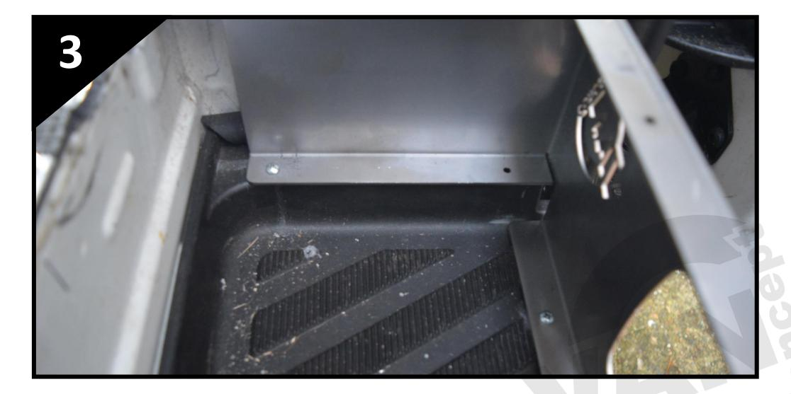
• Screw four pan head screws in the bottom to secure the box in place (two at the rear and two at the front).
