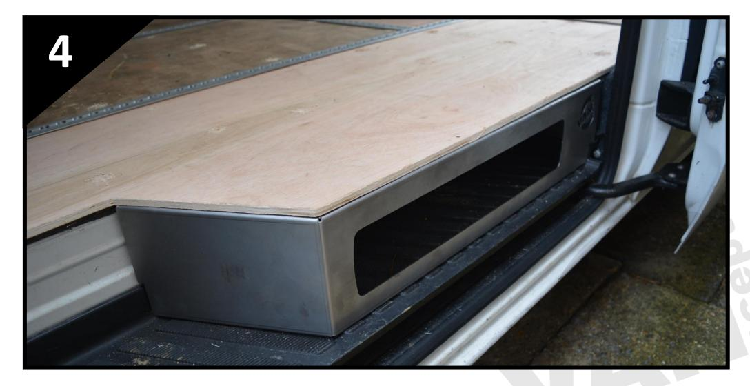
• If fitting a new floor, position your floor in the van and scribe around the box before cutting to the correct profile.
