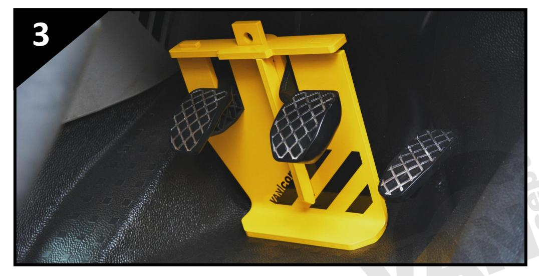
• Fit the top plate over the three tabs on the top, with the circular edge facing forwards. This should fit flush on the top edge of the lock plate and vertical plate.
