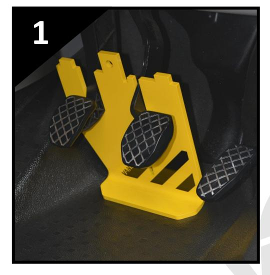
Offer the lock plate into position around the clutch and brake pedal by rotating upwards from underneath.
