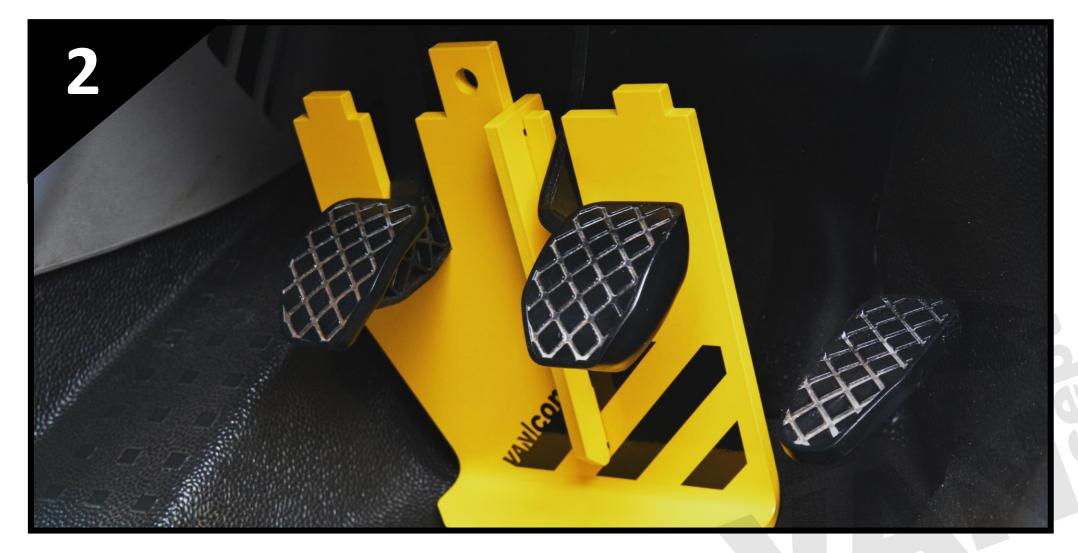
Position the vertical plate through the slot in the lock plate and slide downwards to locate the top hook in position.
