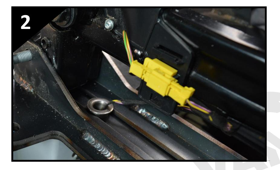
• Disconnect the van battery and wait 20 minutes, before disconnecting the Airbag sensor connector mounted on the central seat rail.
