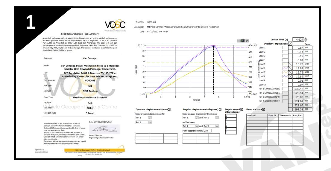
• VOSC Test Certification to confirm our double swivel seat base meets EEC Regulation 14.09 & Directive 76/115/EEC as Amended by 2005/41/EC Seat Beat Anchorage Test for use on the Mercedes Sprinter '18-.
